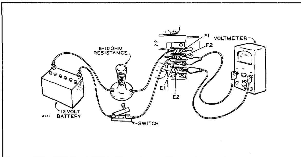
Fig. 4.1 — Flashing the Field See Sect. 4.3.1.1.
