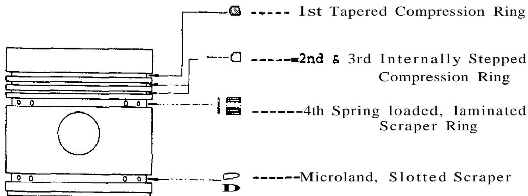
Piston Ring Arrangement Shown Four-107 Engines Rated up to 3000 **RM**
