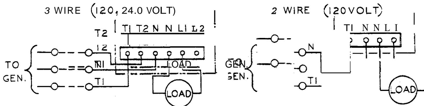
1. Connect DM (Dyna-Monitor) T1, T2, and N to generator junction box as shown above, if not already done.
