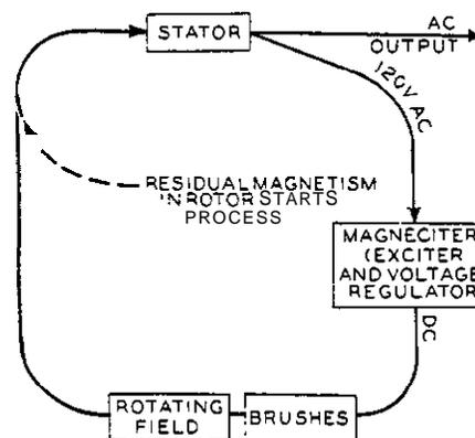
Fig. 4.A — Schematic, Alternator and Exciter
