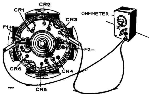
FIGURE 9. TESTING ROTATING RECTIFIERS
