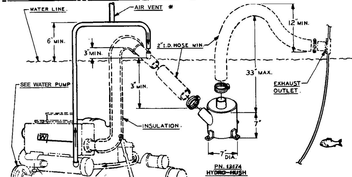
\* AIR VENT MUST BE INSTALLED AT HIGHEST POINT AND ABOVE WATER LINE IN SEA WATER CIRCUIT TO BREAK VACUUM AFTER ENGINE SHUT DOWN, PREVENTING SIPHONING OF SEA WATER INTO ENGINE.
