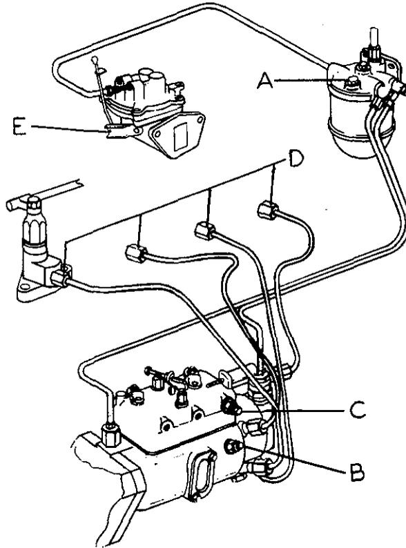
1. Ensure fuel shut **off**, valve is open.
