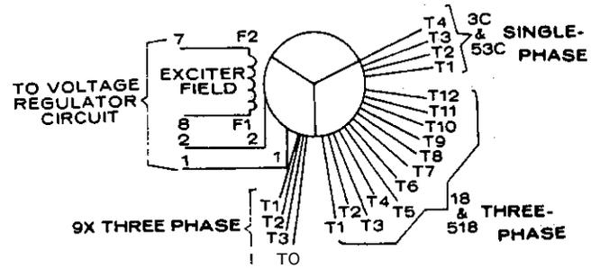
FIGURE 2. SINGLE AND THREE PHASE GENERATOR SCHEMATIC (COMPOSITE)
