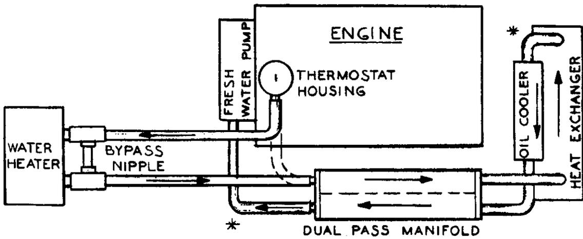
\* ALTERNATE PLACES TO INTERRUPT CIRCUIT AND CONNECT HEATER IN SERIES.
