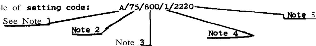
**NOTE 1:** (Prefix indicates pump tested with **BDN12SD12** nozzles) Not required for test purposes. The letter "A" will normally be used to indicate that the pump is tested with **BDN12SD12** nozzles, but in the case of **Perkins** engines different prefix letters will be used. **These** will indicate **BDN12SD12** nozzles as before but in addition will also indicate the engine type to which the pump is fitted.
