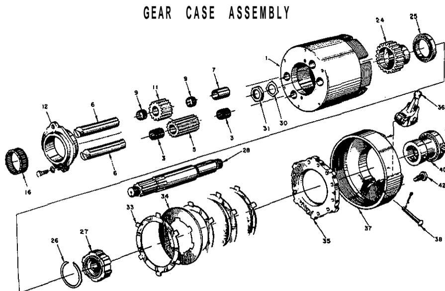
ASSEMBLY OF REVERSE BAND AND YOKE TO GEAR CASE ASSEMBLY
