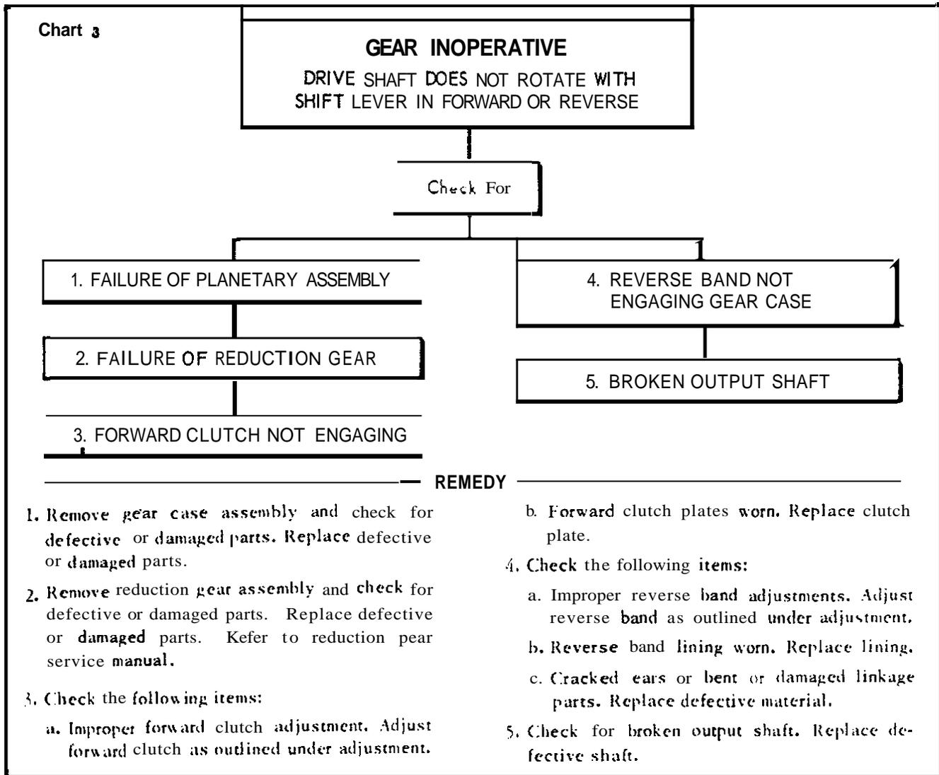
**NOTE:** Disassembly need be carried out only as far as is necessary to correct those difficulties which interfere with proper marine gear operation.
