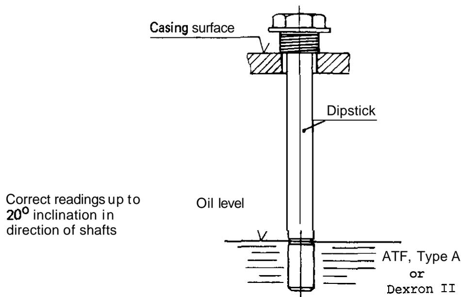
To check the oil level, just insert the dipstick, do not screw in. Retighten the hex screw with the dipstick after the oil level check.
