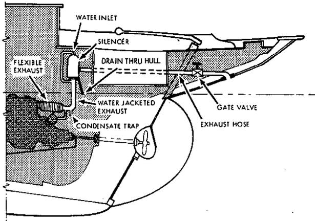
**EXHAUST SYSTEM WITH WATER JACKETED STANDPIPE**
