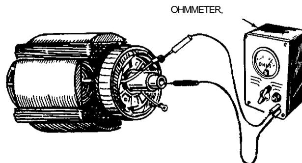
CONTACT ONE PROD TO EACH OF THE FIELD LEADS AND OTHER PROD TO ROTOR SHAFT. IF ROTOR IS GOOD, THERE WILL BE NO READING ON OHMMETER.
