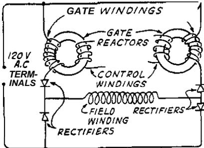
Fig. 4.D — Power Supply with Gate Reactors
