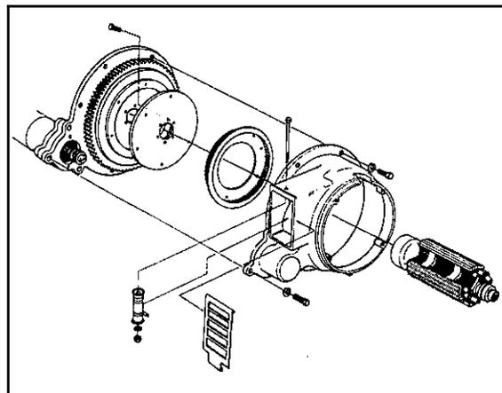
Fig. 4.N — Removing Rotor
