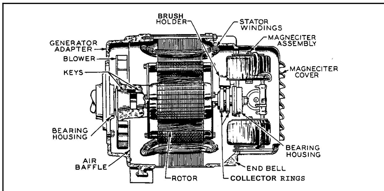
Fig. 4.B — Revolving Field Generator Cross Section
