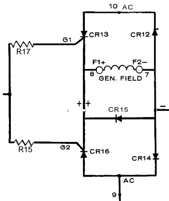
FIGURE 10. SILICON CONTROLLED RECTIFIER BRIDGE
