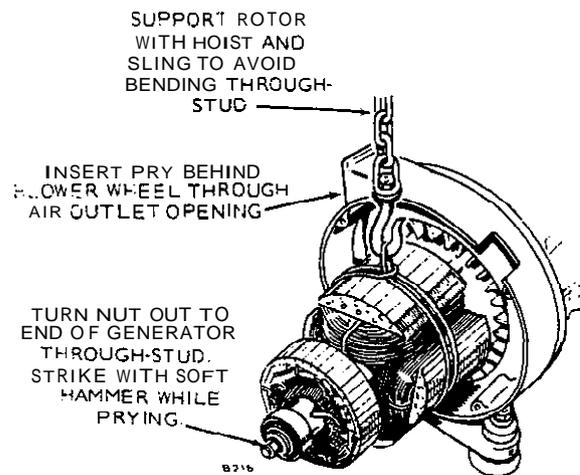
FIGURE 21. ROTOR REMOVAL
