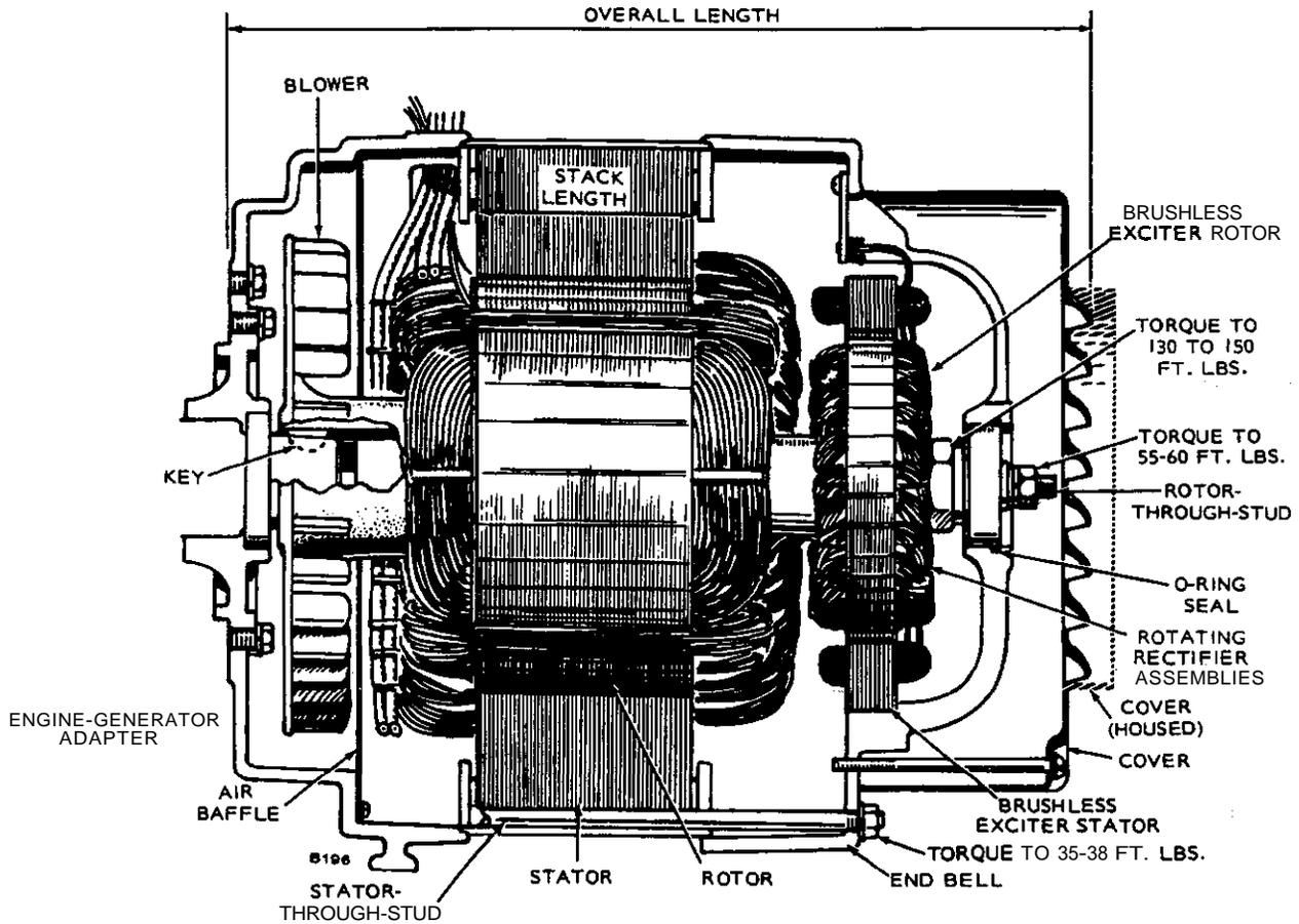
FIGURE 1. GENERATOR (SECTIONAL VIEW)
