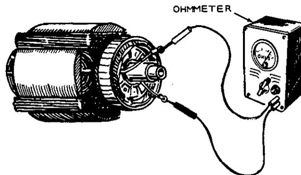
CONTACT ONE PROD TO ONE FIELD LEAD AND OTHER PROD TO OTHER FIELD LEAD. RESISTANCE VALUES ARE GIVEN IN TABLE 2.
