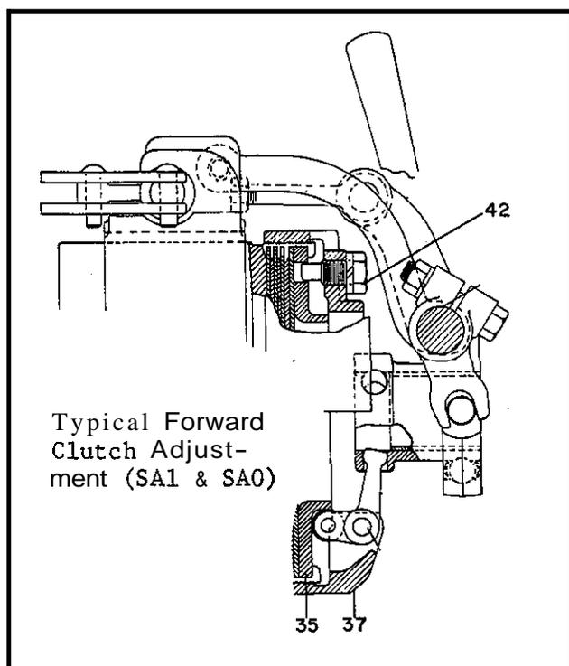
1. Back out the lock screw (42) until the dog on the end of the lock screw is clear of the hole in the pressure plate (35).
