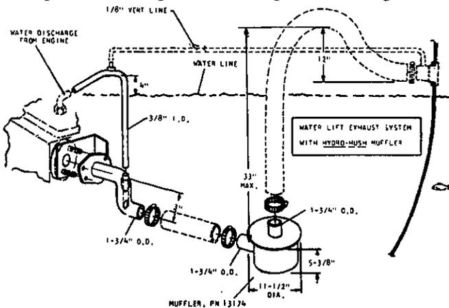
**WATER LIFT EXHAUST SYSTEM WITH "HYDRO-HUSH" MUFFLER**
