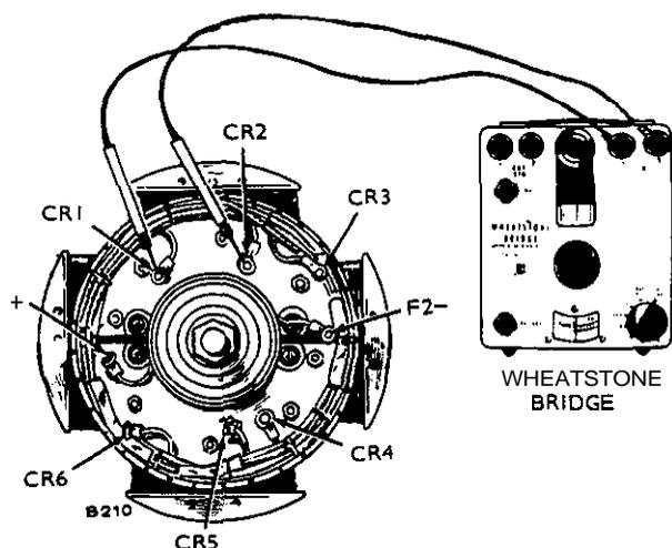
FIGURE 15. TESTING EXCITER ARMATURE
