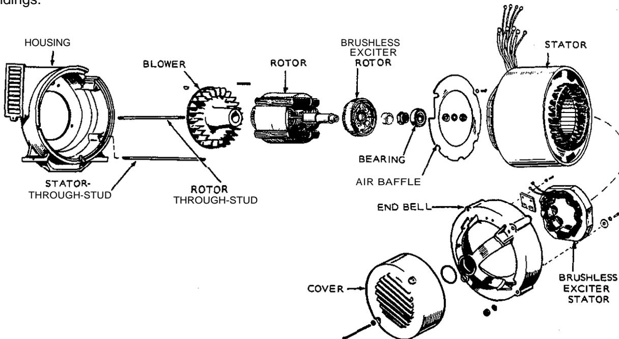
FIGURE 20. GENERATOR DISASSEMBLY
